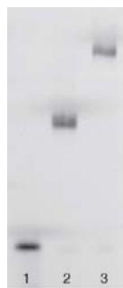
Fig. 6. Native polyacrylamide gel electrophoresis demonstrating cargo binding. When bound to a biotinylated walker, the mobility of 60 kDa streptavidin [8] is greater than that of the 150 kDa anti-biotin antibody [6]. Lane 1: walker. Lane 2: walker bound to streptavidin. Lane 3: walker bound to anti-biotin antibody
